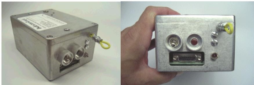
Figure 3.2 Two views of the Industrologic "PDAS" data acquisition unit used in this experimental study.
