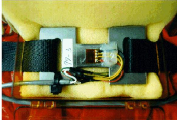
**Figure 3.3 Pictures of the home-made riser load link.**
