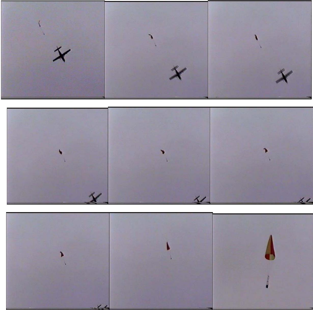
**Figure 3.7 Inflation sequence of the 16ft TCD used during drop YPG034, as filmed from the ground**
