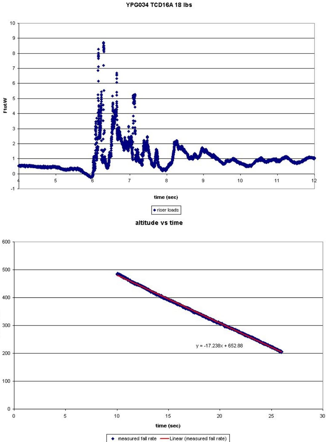
**Figure 3.4 Riser loading and fall rate curves measured during drop YPG034. The lower figure also includes a linear fit to the data. The time on each curve is synchronized. The fall rate curve does not include inflation. Video confirms that inflation ends at  $t \sim 10$  sec.**
