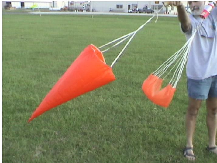
**Figure 1.3** One example TCD used in this study. Note that the the cruciform parachute shown next to the TCD features the same drag area. Note also that the TCD shown has four suspension lines.
